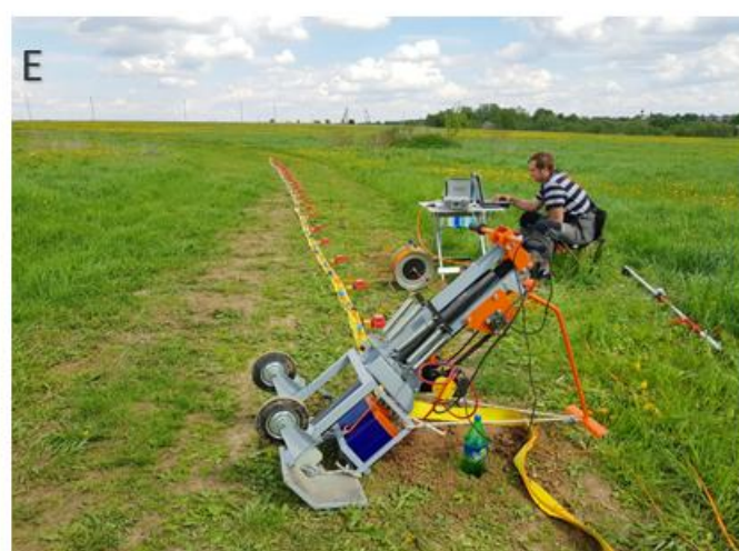
Figure 6: Seismic surveying process and potential impacts. (A) Showing an animated vibroseis process, (B) Showing a real life vibroseis process, (C) Showing minimal dust generated from the process, (D) Showing minimal vegetation impact associated with a new access path (transect route), (E) Showing the weight drop alternative method and (F) showing magnetotelluric survey
